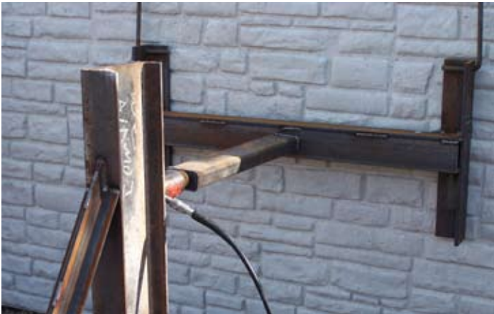
Fiber-reinforced Verti-Crete fence panels were tested for strength by applying horizontal pressure in incremental amounts with a hydraulic jack.
